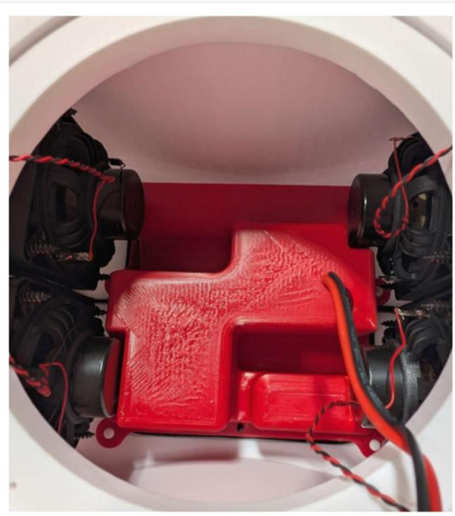
20) Prepare the Tang Band W3-2052SC 3" RBM Neodymium Subwoofers for wiring by cutting off the included 2-pin plugs and then stripping about 0.75" of insulation off of each wire. Also, strip about 0.75" of insulation off the output (red/black) wires from the SA25 Plate Amplifier.
