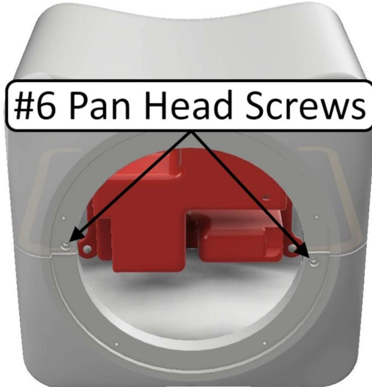
12) On the back of the enclosure, insert 2 x #6 x 3/4" Pan Head Deep Thread Black Screws (E) into the holes shown below. Tighten these screws fully and ensure the head of the screw is completely countersunk below the amplifier mounting surface.
