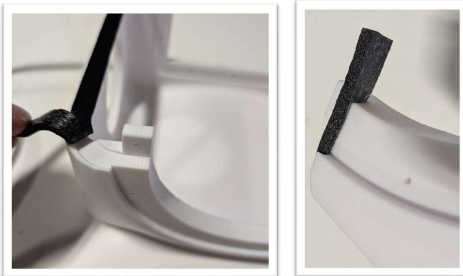
4) Use a sharp knife to cut the ends of the gasket tape flush with the edges of the enclosure as shown.
