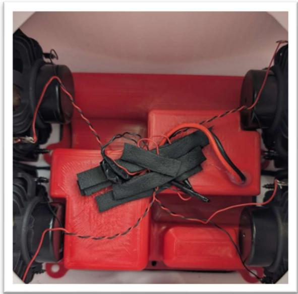
**24)** Prepare the **Dayton Audio DS175-PR 6-1/2" Designer Series Passive Radiator (C)** for installation by adding the five **1/4" x 1" Zinc Fender Washers (G)** to the back side of the passive radiator. Secure the fender washers with the screw and washer provided in the DS175-PR Passive Radiator package.
