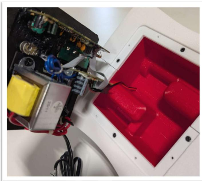
**17)** Secure the SA25 Plate Amplifier to the enclosure with **8 x #6 x 3/4" Pan Head Deep Thread Black Screws (E)**. Carefully tighten the screws to avoid stripping the screw holes. As you tighten these screws, they will pull the Amplifier Cover into place creating a tight seal to the enclosure.
