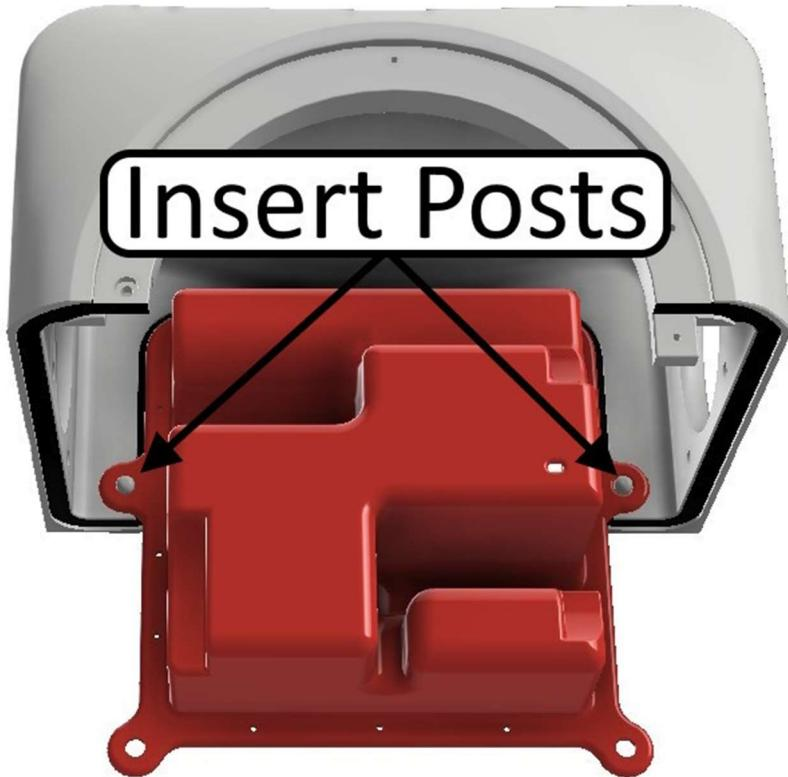
8) Insert 2 x #6 x 3/4" Pan Head Deep Thread Black Screws (E) into the holes shown below. Tighten the screws *just* until the Amplifier Cover compresses the gasket and is pulled flush with the top piece (do not overtighten the screws). The screws should be completely countersunk below the amplifier mounting surface.
