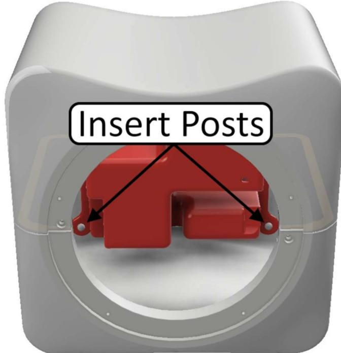
10) Compress the gasket by carefully pressing the front of the Top and Bottom Pieces together while ensuring that the tabs are inserted into their corresponding notches.
