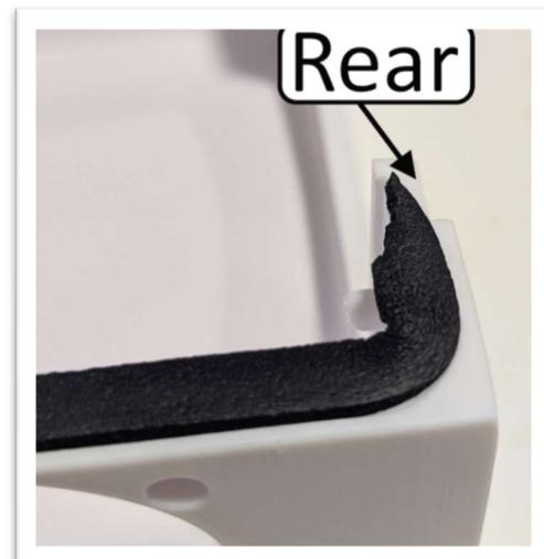
5) Apply the 14" pieces of gasket tape to the Amplifier Cover mounting surface (both Top and Bottom Pieces) in the grooves provided. Leave approximately 1" extra material on each end. Press hard to ensure the tape has adequate adhesion to the mating surface, especially around the curves. Also, do not stretch the gasket tape as you apply it to ensure proper adhesion.
