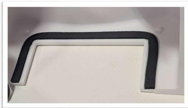
6) Use a sharp knife to cut the ends of the gasket tape flush. For the Bottom Piece the tape should be flush with the edges of the enclosure. On the Top Piece, overlap the gasket you previously applied and trim it flush with the existing gasket.
