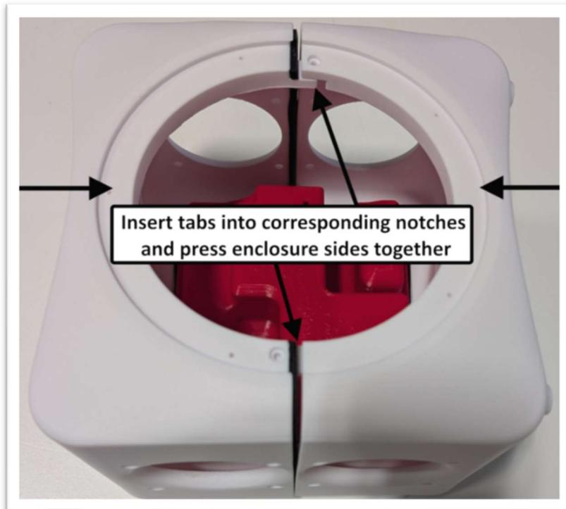
11) Once the tabs are fully seated, insert 2 x #6 x 3/4" Pan Head Deep Thread Black Screws (E) into the holes shown below. Tighten these screws fully making sure the head of the screw is completely countersunk below the mounting surface of the passive radiator.
