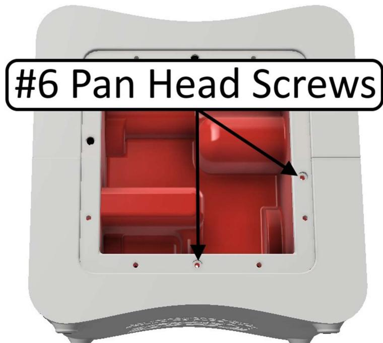
**13)** Carefully tighten each screw to ensure they are fully seated. Also, make sure that the Amplifier Cover is pulled tightly to the Top and Bottom Pieces near each of the 4 screws (there may be some small gaps away from the screws, these will be sealed up when the amplifier is installed)
