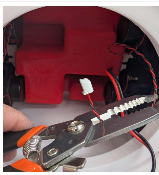
**21)** Push the output (red/black) wire from the SA25 Plate Amplifier back into the hole in the Amplifier Cover until only 6" - 8" remain inside the enclosure. Seal the hole and secure the wire using a little bit of hot glue (caulk, epoxy, museum putty, or even poster tack will work also).
